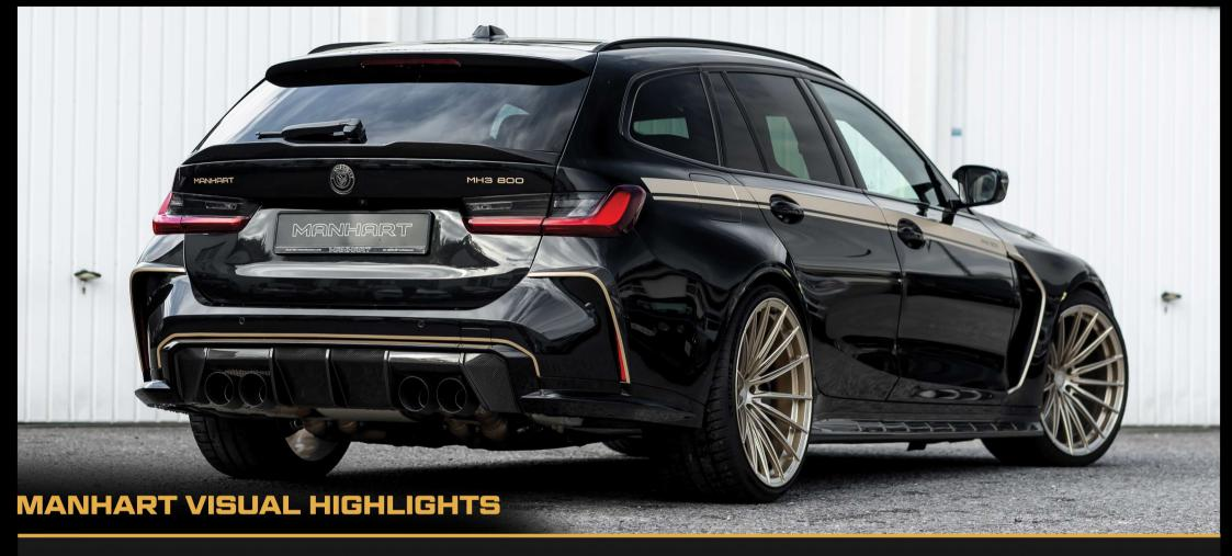
Last but not least, the MH3 800 Touring is fitted with a complete kit of MANHART carbon add-on parts. New radiator grille kidneys, a front spoiler, a two-piece apron attachment and a bonnet. MANHART customised the side section with attached side louvres on the front wings and sills. At the rear, side skirt attachments and a carbon boot spoiler round off the package.
